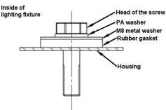
They are to be used as on pictures above. Tightening torque of the screws must not exceed 1Nm so the gaskets won't be significantly deformed.
