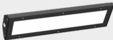
Vandalproof light fitting with LED modules, designed for corner mounting as one of LINE system modules. Behind of housing is a gap for routing cables of surface-mounted electrical installation. Very high impact resistance factor (IK10+) is achieved thanks to stainless steel housing and thick polycarbonate diffuser.
