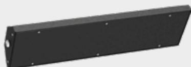
Stainless steel, vandalproof blinding plug used as a distance between other modules. Available in different lengths. Designed for corner installation as module of LINE system. Behind back of housing is a gap for routing cables of surface-mounted electrical installation.
